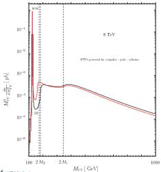
Peculiar structure of the signal distribution: enhancement of the H(126) cross-section in the high mass region
