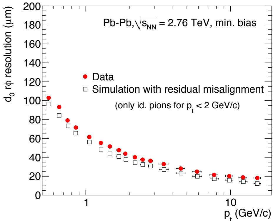
Track impact parameter resolution  $\sim 60\mu\text{m}$  for  $p_t = 1$  GeV/c
