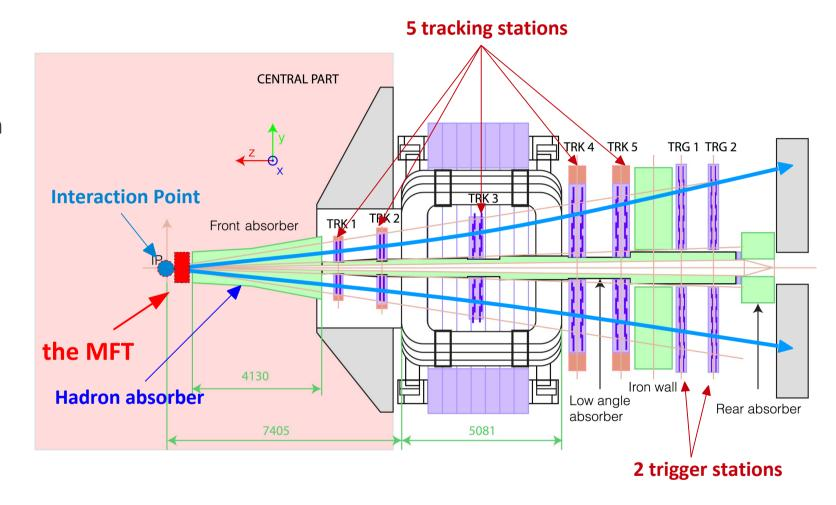
**Non-trivial integration challenges:** constraints from the upgraded ITS, the future beam pipe, the existing hadron absorber, . . .  $\rightarrow$  See talk by G. Batigne
