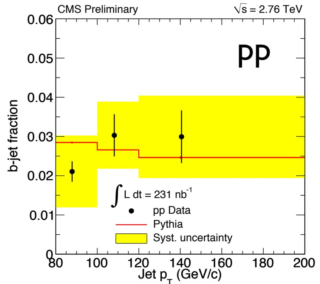
$$\text{b-jet fraction} = N_{\text{jets}}^{\text{tagged}} * \text{purity/efficiency}$$
