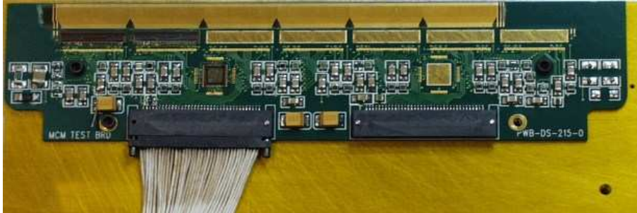
Fig. 3.14 - Picture of a mini-MCM (see Chap. 7) during assembly; only the left GTRC and the first two GTFEs are in place.
