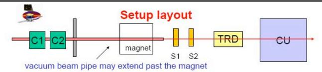
C1-C2: Cherenkov counters S1-S2: trigger scintillators
