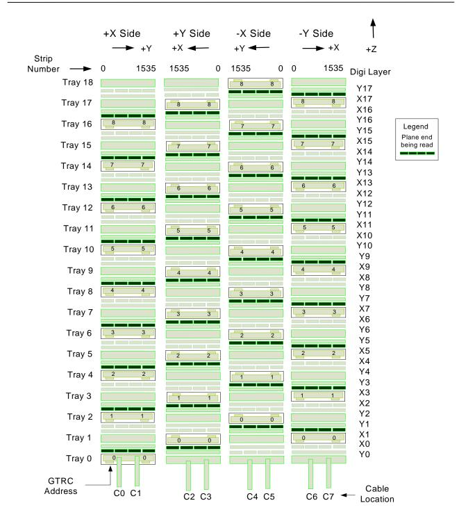
Figure 12: The Four Sides of the TKR Tower with Cables. "X" or "Y" Means Measured Coordinate.
