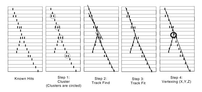
Figure 24: Four Steps of TKR Reconstruction (Illustrated)
