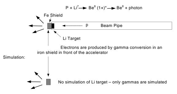
Figure 27: Simulation of VDG Gammas – Simulated Particle Source Generation
