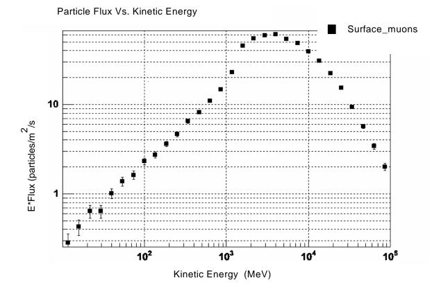
Figure 28: Particle Flux vs. Kinetic Energy for surface\_muon Source
