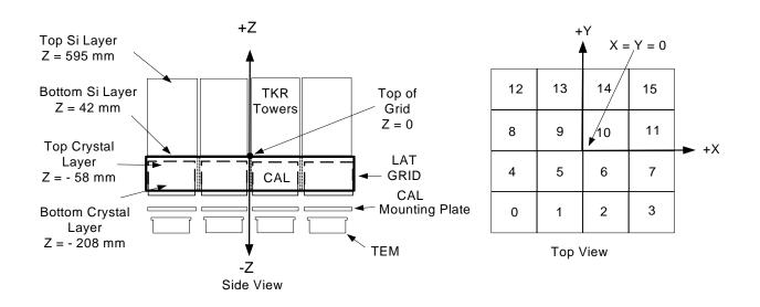
Figure 5: LAT Tower Numbering and Grid Coordinate System
