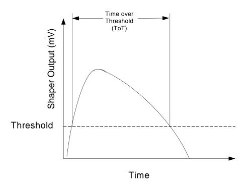
Figure 20: Shaper Output Time over Threshold
