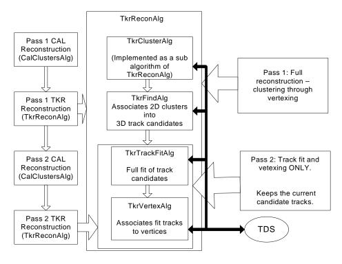
Figure 25: Iterative TKR Reconstruction Algorithms (Block Diagram)
