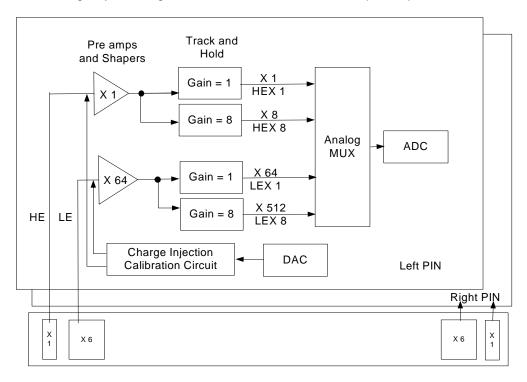
Figure 13: CAL FEE Simplified Schematic Diagram
