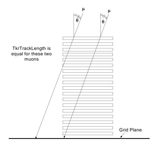
Figure 29: TrkTrackLength Example of Easily Misinterpreted Data
