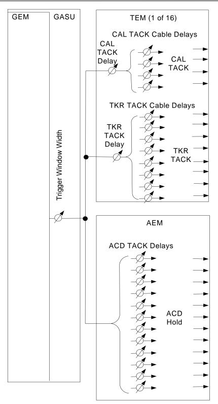
Figure 18: Conceptual Trigger Delay Adjustments Diagram (GEM Outputs)
