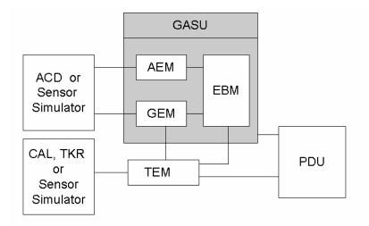
Figure 2: Principal LAT Components (Block Diagram)
