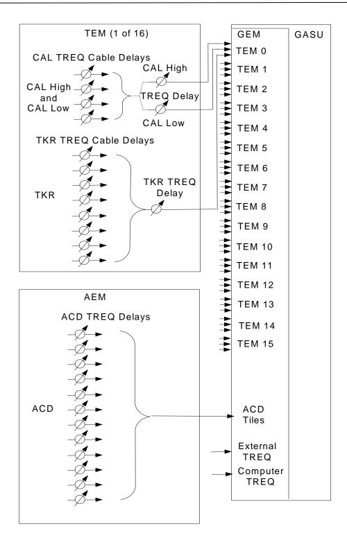
Figure 17: Conceptual Trigger Delay Adjustments Diagram (GEM Inputs)
