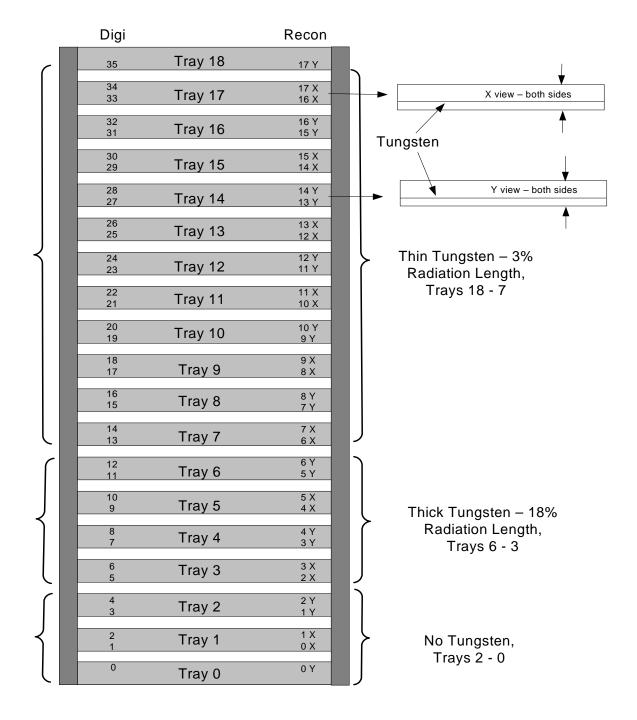
Figure 6: TKR Tower Numbering Scheme.
