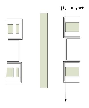
Figure 30: A Charged Particle's Path is Parallel to the Z Axis and only Strikes Every Other Crystal
