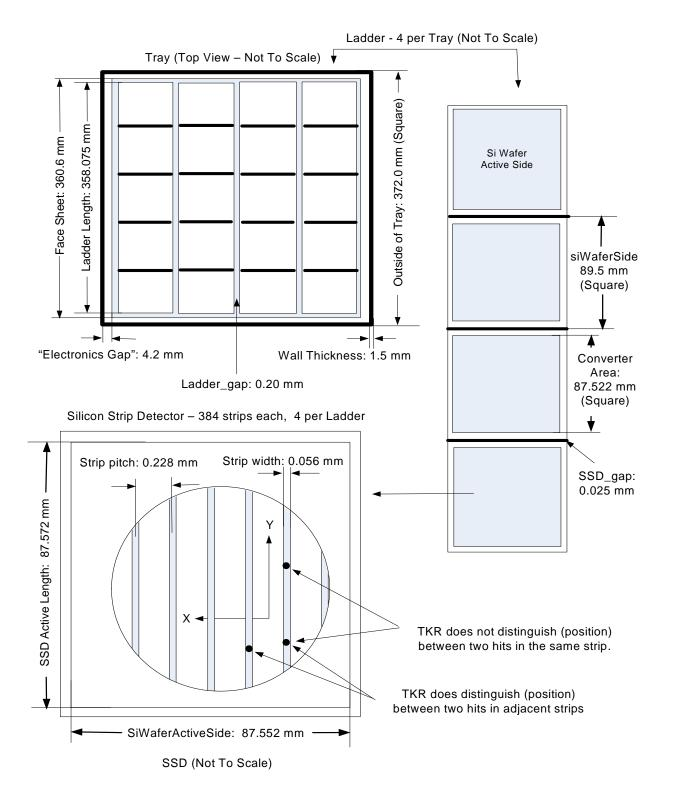
Figure 7: TKR Plane Physical Details (X-View)
