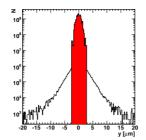
Figure 2: Transverse beam profiles at the BDS entrance.
