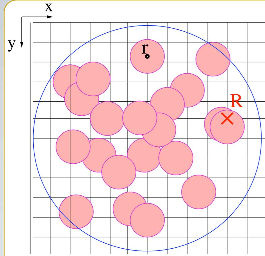
1. Generate configurations for the positions of nucleons in the transverse plane ( $r_i, i=1\dots A$ ). Wood-Saxons thickness function  $T_A(\mathbf{R})$
