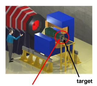
CHIC: Vertex detector located 7.5 cm downstream of the target (7 cm for NA60)
