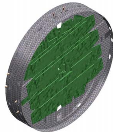
Drawing Of forward Microstrip tracker
