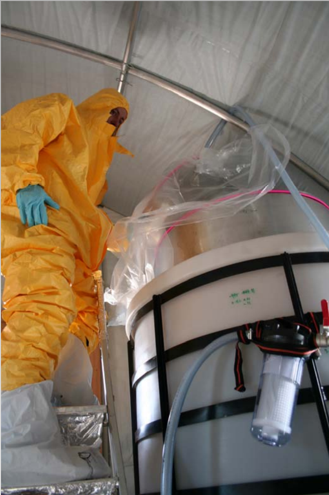
DOME C snow is melted in a dedicated double-tank and gravitationally sieved
