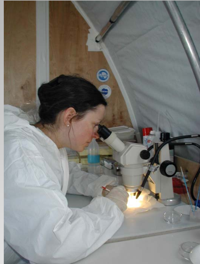
The 30 \mu\text{m} filters are pre-analyzed in a mini-lab to control terrestrial contamination
