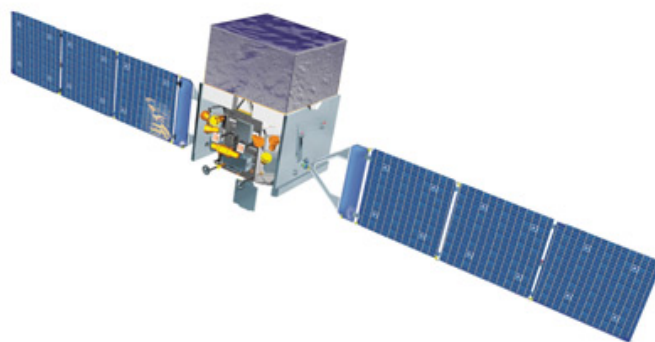
Figure 2.2: Fermi spacecraft with two instruments on board: the Large Area Telescope and the Gamma-Ray Burst Monitor. Image courtesy: NASA.
