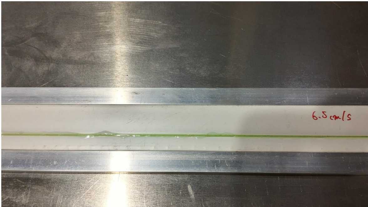
Figure C.2 – Scintillators after the gluing procedure. The amount of optical cement has been dispensed uniformly over the fiber.
