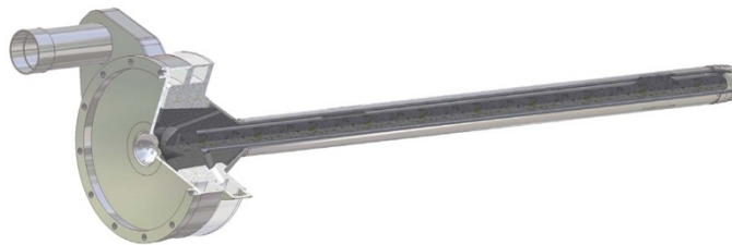
Figure 2.4 – Scheme of the carbon target installed in the beamline.
