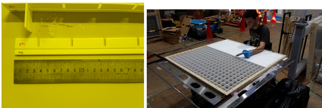
Figure 2.20 – (a) Scintillators used to build the grid structure of the Water Module. (b) Gluing of 40 scintillators to form a plane on the grid structure.
