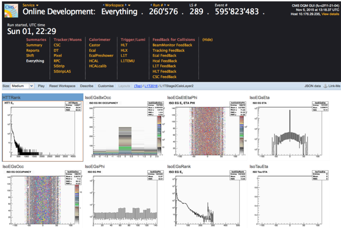
Figure 3.16: Sample of distributions available in the online DQM of the Level-1 Calorimeter Layer-2. On the top row, from left to right: the distributions of L1 HTT, the 2D distribution of the E_T of L1IsoEG candidates as function of the bunch crossing, the E_T -weighted 2D distribution of the \eta - \phi position of L1IsoEG candidates and the \eta distribution of L1IsoEG candidates. On the bottom row, from left to right: the 2D distribution of the \eta - \phi position of L1IsoEG candidates, the \phi distribution of L1IsoEG candidates, the E_T distribution of L1IsoEG candidates and the \eta distribution of L1Tau candidates.
