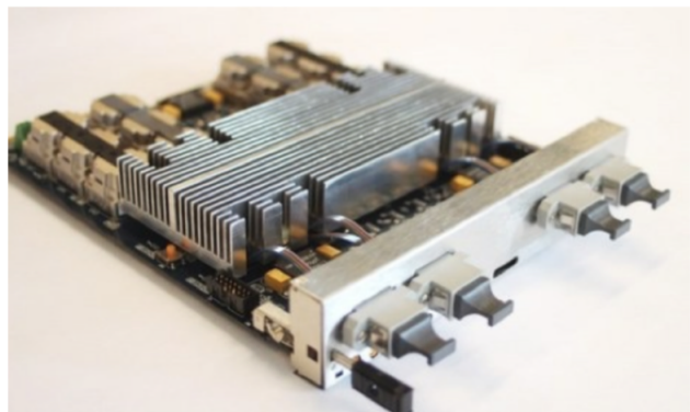
Figure 3.5: CTP7 [142] (left) and MP7 [143] (right) boards used in the upgraded CMS Level-1 Calorimeter Trigger.
