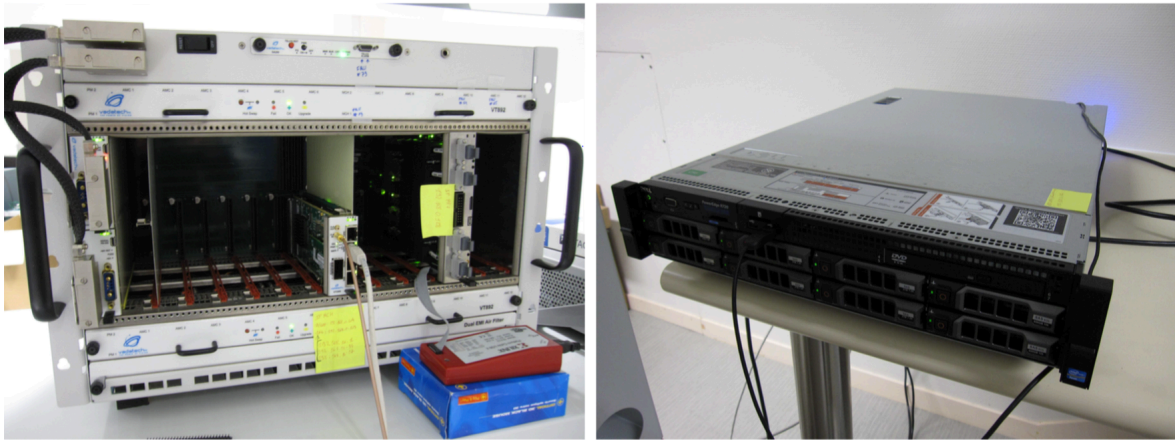
Figure 3.13: \mu TCA testbench used at LLR. On the left, the Vadatech \mu TCA crate, with the MHC board in the middle of the crate (used to download firmware) and the MP7 board on the right of the crate. On the right, the Dell computer used for the compilation of VHDL programs and the production of FPGA firmwares. [140]
