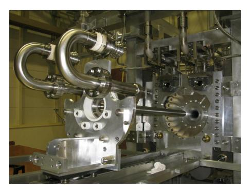
Figure 2.9: The T2K target inserted in the first horn.
