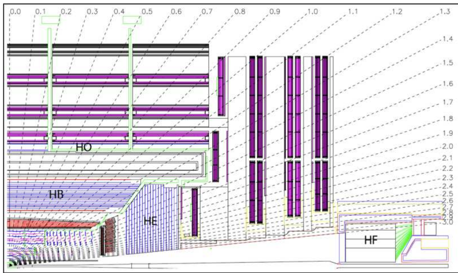
Figure 3.11: Longitudinal view of the CMS hadron calorimeter and its sub detectors : Barrel (HB), Endcap (HE), Outer (HO) and Forward (HF) calorimeters.
