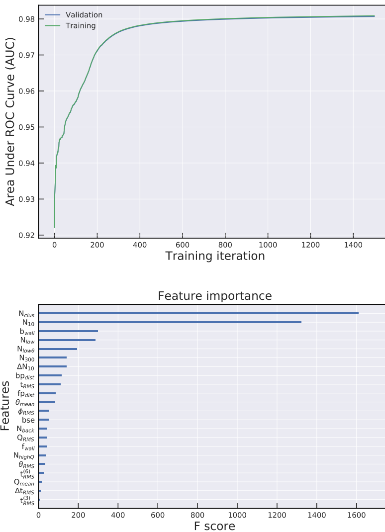
FIGURE B.1: Top: evolution of the model performance metric ( 1 - AUC ) as function of the training iteration. The model improves sharply in the first 200 iterations, and begins plateauing after around 500 iterations. The performance on the training set (green line) and validation set (blue line) are both plotted. In practice, the two lines coincide almost completely due to the limited amount of overtraining. Bottom: relative importance ranking of each of the observables used by the BDT. Higher importance implies that the observable is used more often, and to make more powerful domain splits.
