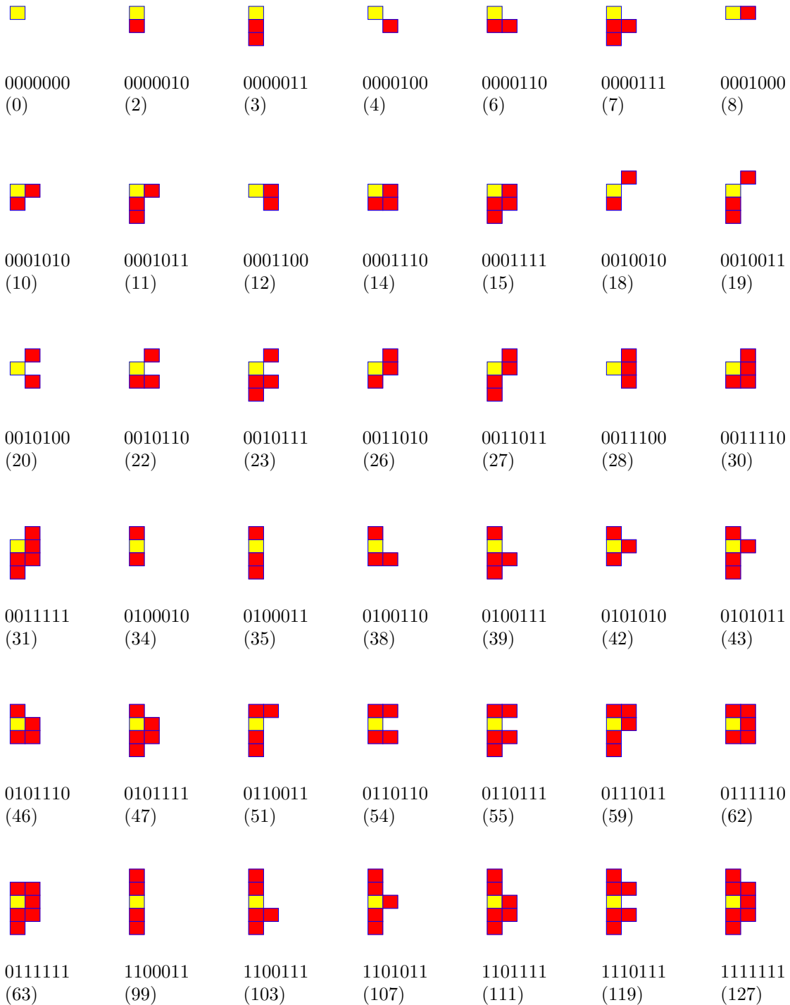
Figure 3.18 – Overview of the 42 symmetric shapes of a L1 \tau_h cluster. Each square denotes a TT, and the yellow one denotes the seed of the cluster. The number below each shape represents its binary representation in the format discussed in the text and its conversion in decimal format is reported below between brackets for an easier comparison with the other figures.
