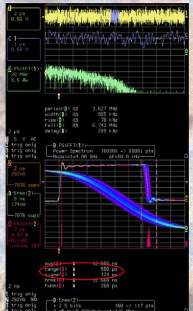
40 Mhz clock with injected jitter
