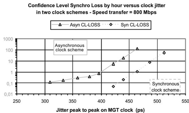
Figure 6 : Synchronization loss measurements
