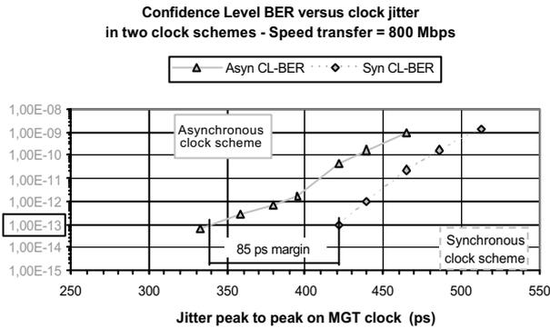
Figure 5 : BER measurements
