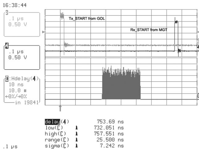
Figure 7 : Latency delay distribution in the asynchronous mode
